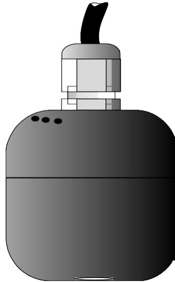
The OxyGuard Probe is a membrane covered galvanic cell that generates an electrical signal proportional to the oxygen pressure it senses, no matter whether it is in water, air, gas, wine, oil or something else. The probe can be used to measure dissolved oxygen in aquaculture, the environment, in clean water, waste water and in oil or other fluid. It can measure very small oxygen concentrations in inert or explosive gases as well as the oxygen content of ambient air and the purity of oxygen gas.
