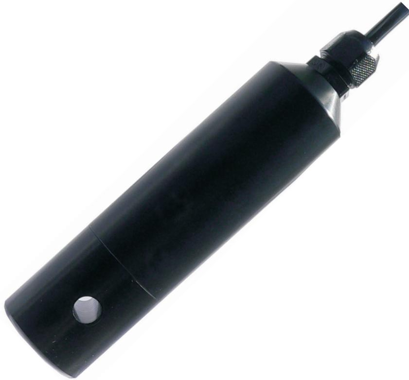
The OxyGuard Salinity Probe is specially designed for aquaculture use. Factory calibration and automatic temperature compensation make it very easy to use. It is found in two versions. One is a 3-wire 4-20 mA sensor - connect it to 24 VDC and the output varies between 4 and 20 mA according to the salinity. The other has data bus connection for use with OxyGuard Pacific.
