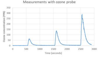
Graph of response time: At 550 seconds a portion of ozone was added and the sensor responds almost immediately. At 1550 and 2490 seconds, the same was done with increasing portions of ozone. The fast break down of the ozone is obvious as well
