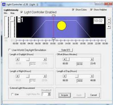
Commander has an artificial daylight program. This can control fluorescent or LED lamps with analogue or DALI signals.
