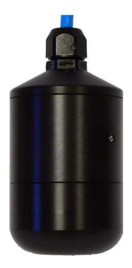
The Model 420 is a membrane covered galvanic oxygen probe with built-in two-wire 4-20 mA transmitter. The probe is connected to a DC supply and draws a current of between 4 and 20 mA corresponding to the oxygen concentration.
