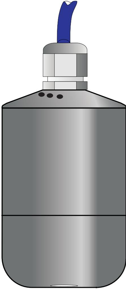
The Model 420 is a membrane covered galvanic oxygen probe with built-in two-wire 4-20 mA transmitter. The probe is connected to a DC supply and draws a current of between 4 and 20 mA corresponding to the oxygen concentration.
